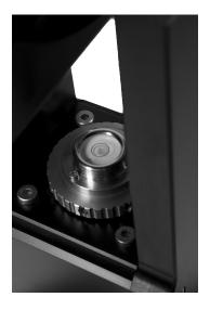
Before you begin to assemble the arm sections, you should level the fulcrum. The fulcrum has a level on the tie down bolt.
