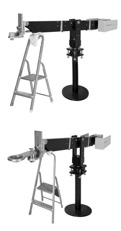
Balance the arm by putting some weight in the bucket, but maintain downward force on the support in the front end.
